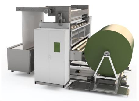
The textile first passes through the dyeing station where the dye dispersion is applied normally at between 0,5 to 0,9 litre/ kilo depending on fibre type and fabric construction.
